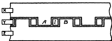
FIG. 195.—The Fleming-Clinton Commutator ; the Surface laid out flat.
