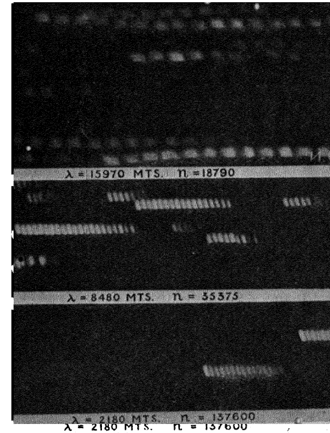
FIG. 234.—A Half-Size Reproduction of three Spark Photographs, the Oscillation Frequencies being 18,790 per sec., 35,375 per sec., and 137,600 per sec.
