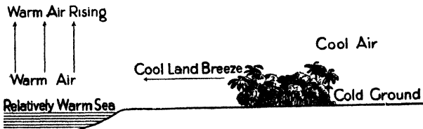
FIG. 21.—Diagram showing the cause of a land breeze by night.
