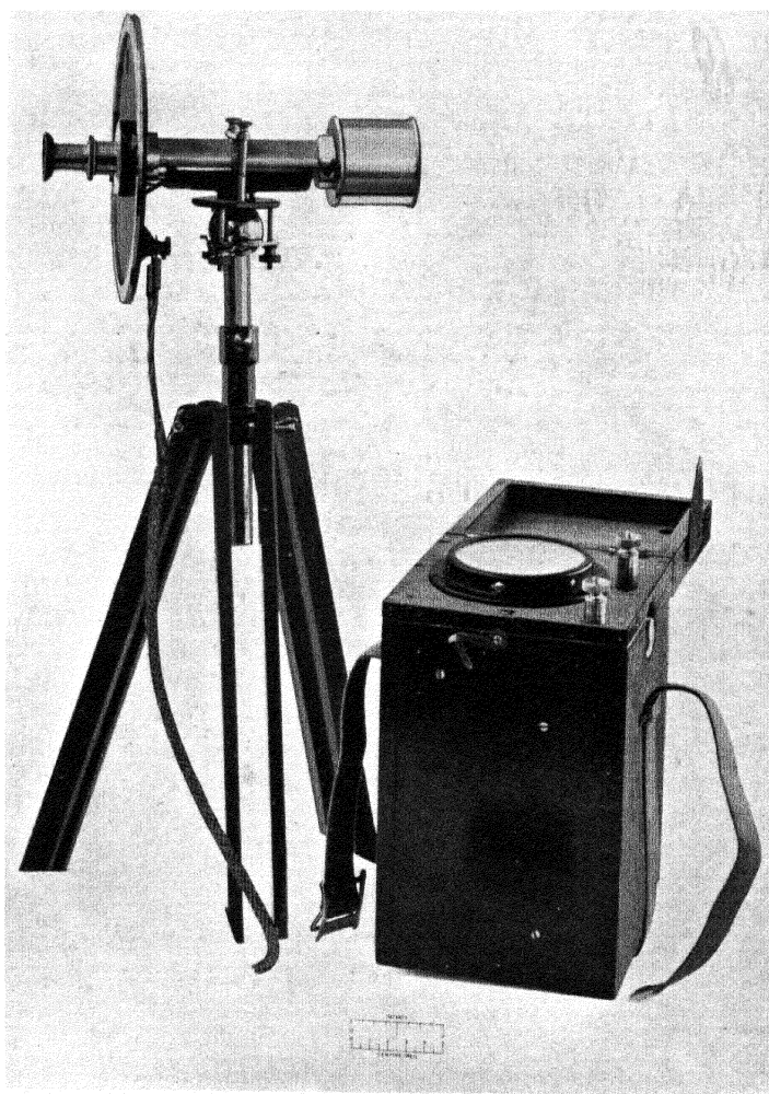
Fig. 147.—Cambridge Optical Pyrometer (With case for battery, &c., for the standard comparison lamp)
