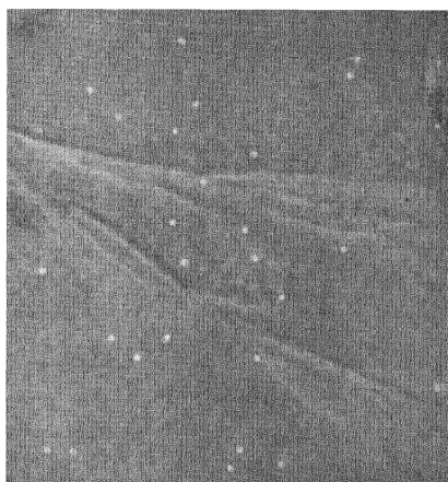
FIG. 2 Tick marks on a piece after it has been tanned
