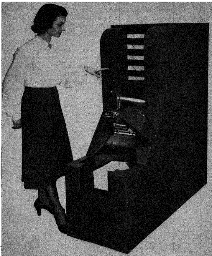
In most sales promotion departments there is considerable gathering to be done. This Thomas collator gathers 1,500 sets of papers an hour and automatically stacks them crisscross for stapling.
