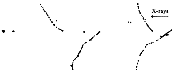
FIG. 8. Long tracks with large forward component. Sphere tracks. Cylindrical X-ray beam, 0.5 mm. in diameter, has traversed 8 \times 10^3 cm. copper. Final pressure 19 cm.
