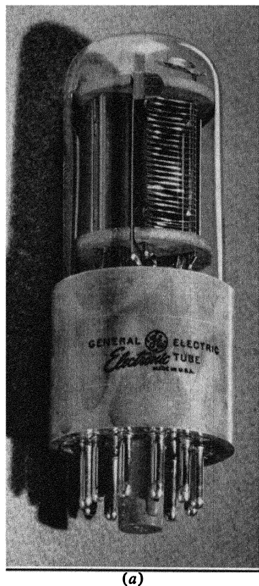
FIG. 4. Photomultiplier tube. a. Photograph. (Courtesy of General Electric Co.) b. Schematic diagram.
