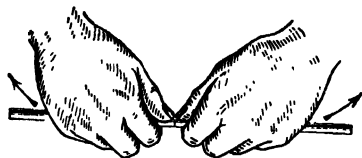
Fig. 28. Position of hands when breaking scratched glass tube
