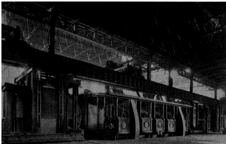
FIG. 103. A 400-ton active mixer.
