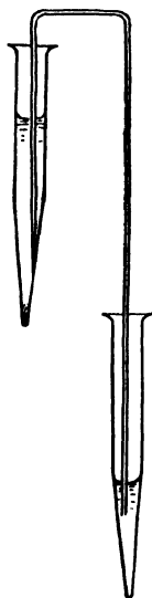
FIG. 17. Separation of precipitate and solution by means of a capillary siphon.
