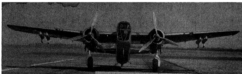
A-20-A LIGHT (ATTACK) BOMBER WITH FOUR CHEMICAL SPRAY TANKS BENEATH WINGS
