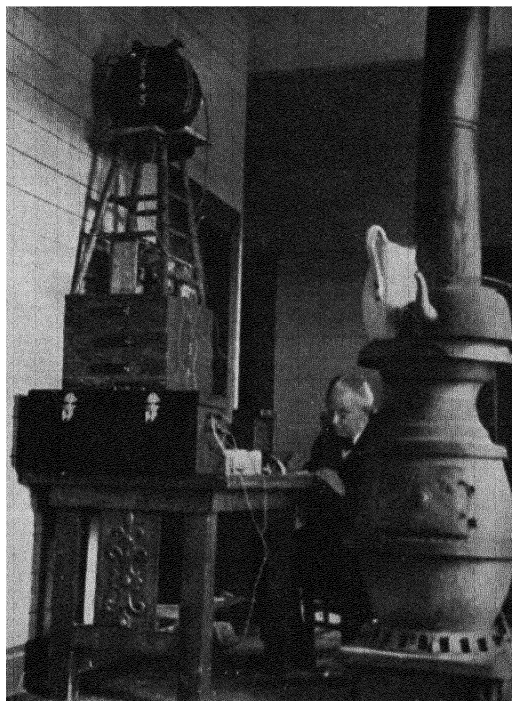
FIG. 60. A cosmic-ray electroscope incased in a spherical lead shield in position in a building on the summit of Pike's Peak. The electroscope is placed near the ceiling of the room in order that radiations from the surrounding soil and rocks may be reduced to a minimum. The observer is Dr. R. A. Millikan.
