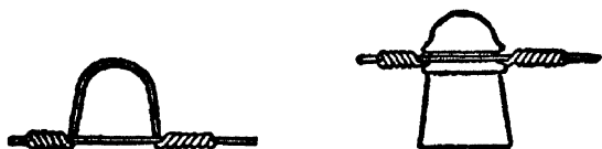
Transmission wire on glass insulator
