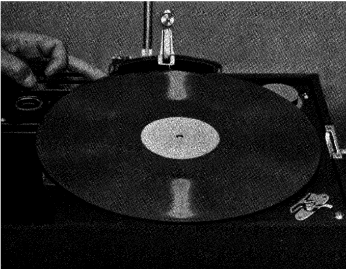
Calibration of a gliding note record by an optical method (Buchmann and Meyer). See p. 51
