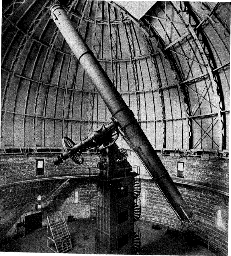
FIG. 2.10. Forty-Inch Refracting Telescope, Yerkes Observatory. The largest refracting telescope; its objective, a pair of lenses 40 inches in diameter at the top of the tube, focuses the light by refraction. This is an equatorial telescope. It can be turned parallel and perpendicular to the celestial equator. Graduated circles on the two axes facilitate the pointing of the telescope to any desired right ascension and declination.
