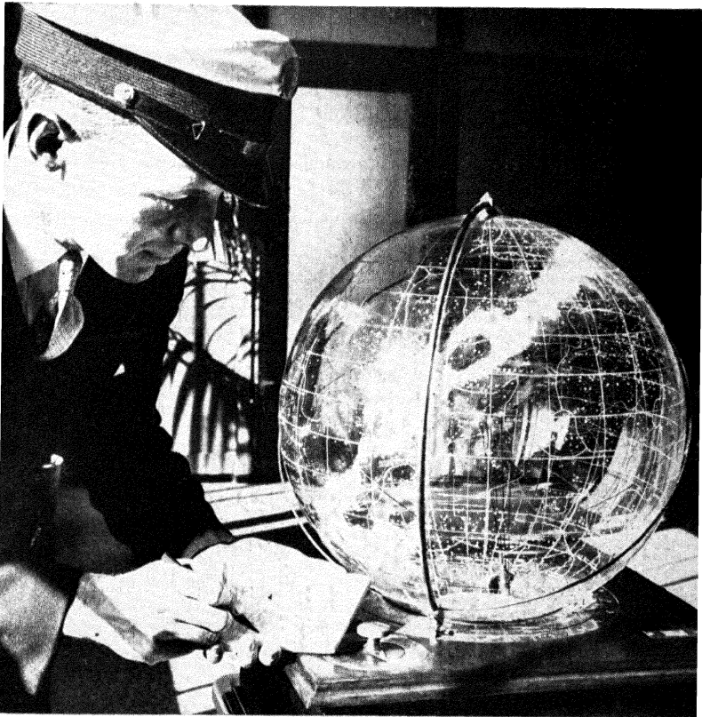
FIG. 4.9A. Transparent Celestial Globe on the Observation Roof of the RCA Building, Rockefeller Center, New York. Inside the globe there are representations of the earth and bright planets; these are supported by thin metal rods in such a way that they can be set at any time in their correct places relative to one another and to the constellations. (By courtesy of Rockefeller Center, Inc.)
