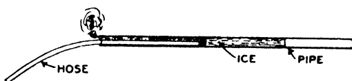
FIGURE 11-3.—The steam hose may be extended up large sized pipe to the ice.
