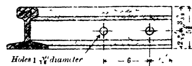
END OF RAIL Showing Fishbolt holes.
