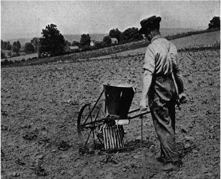
FIG. 13.—A hand fertilizer distributor. Delivery may be concentrated or scattered by moving the tubes.
