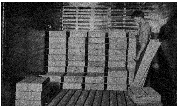
FIG. 129.—Packing crates in the car for shipment. Each crate is held in place by laths nailed to the top. About 600 crates are placed in each car.
