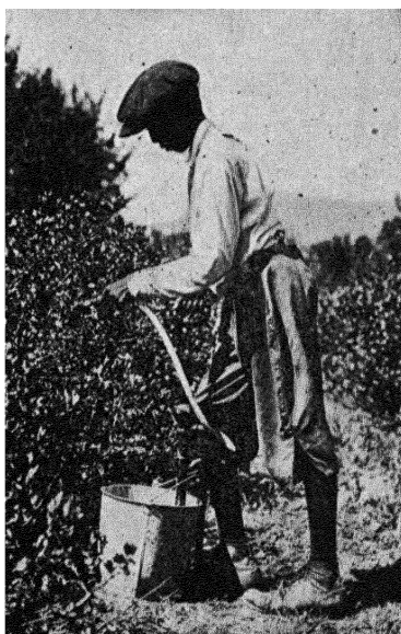
FIG. 18.—Bucket pump. A simple but efficient little pump for small operations. Unhandy to move about.
