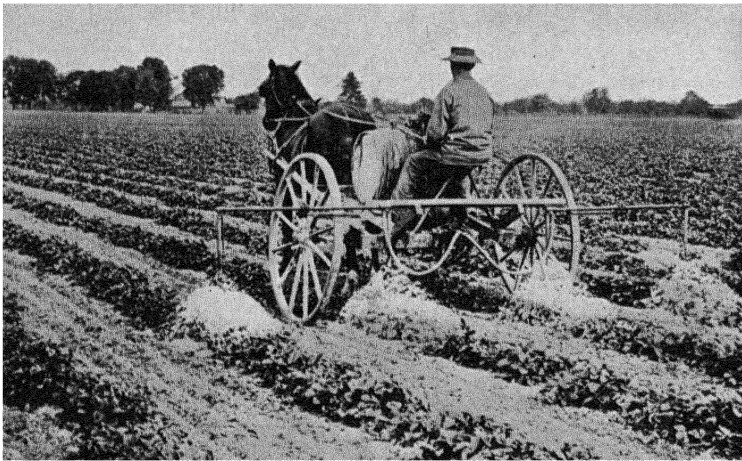
FIG. 20.—Special sprayer for use in strawberry fields. It is a traction type, the power being generated by the turning of the wheels.
