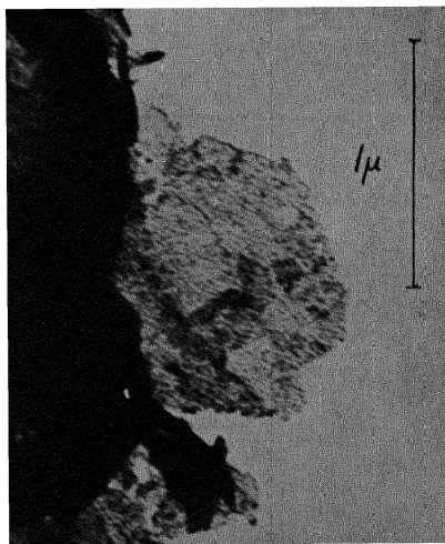
Fig. 9.—Extra-light magnesia from magnesium carbonate.
