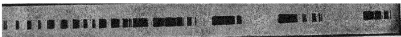
Fig. 10.5b. Spectra of molecular nitrogen. (From Harrison, Lord, and Loofbourow, Practical Spectroscopy , Prentice-Hall, 1948.)
