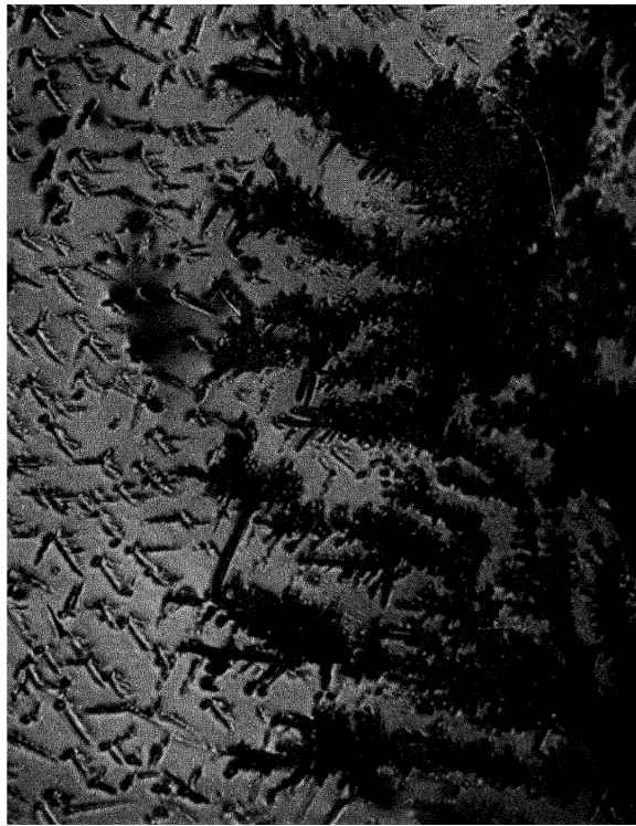
1. Unique fractograph of molybdenum metal showing the external surface of a grain—the grain boundary—with two intruding growths which strongly affect the forgeability. The upper field has feathery forms which are carbides necessary for forgeability. The lower field has a weedy-looking growth of oxide, caught in the act of invading the carbide area to form carbon oxide gas which is removed by the vacuum treatment. The oxide growth causes the grains to fall apart, preventing forging. Magnified 385 times.
