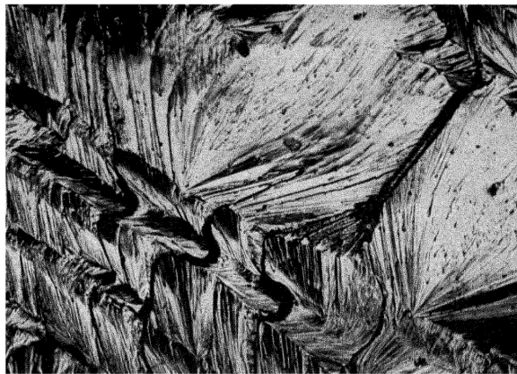
2. Fracture passing through a grain of molybdenum reveals a remarkable pattern which is probably the frozen record of the story of solidification and growth. Magnified 75 times.
