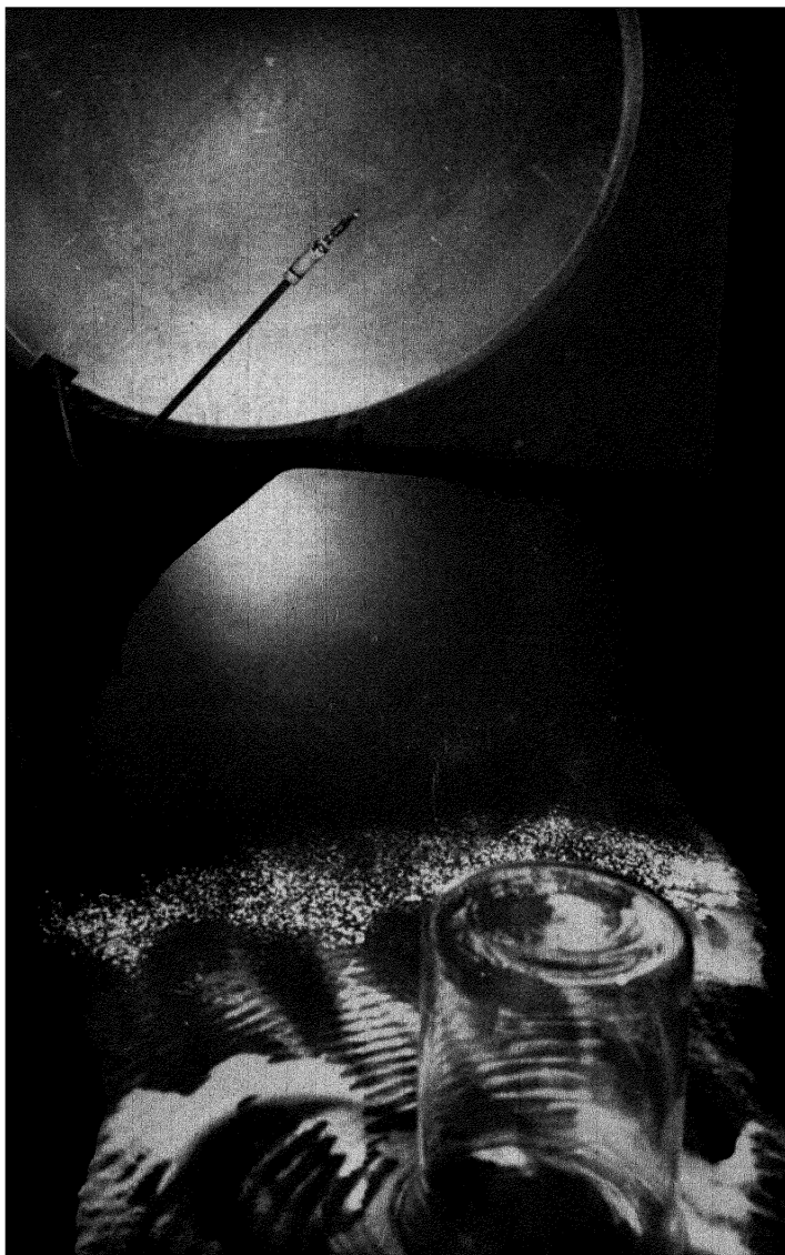
Ultrasonic waves, coming from the tiny whistle on the end of the J-shaped tube, are reflected onto the table by the concave metal disk. The ridges, formed in talcum powder, show the standing waves formed by reflections from the table top and beaker. Courtesy General Electric Co.
