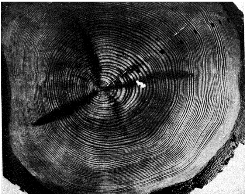
Fig. 70. The cross-section of a beam of Douglas fir, shewing the variations of climate from A.D. 1073, when the tree started to grow, until A.D. 1260, when it was felled. Subsequently to A.D. 1260, the log was used as a beam in a dwelling, which afterwards fell into ruins. The beam was unearthed and studied in 1933, and is of value as filling in the weather record of the two centuries of its growth.
