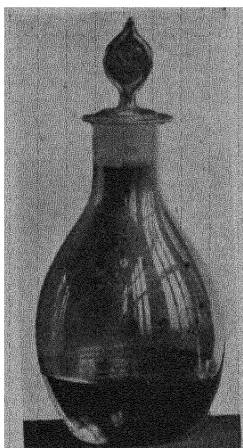
FIG. 36.—FLASK USED FOR ACETONE AND BROMINE TESTS OF WOOD-NAPHTHA.
