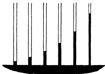
FIG. 126.—Rise of water in capillary tubes.
