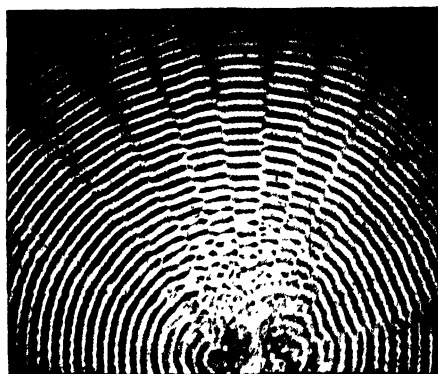
FIG. 213.—Interference of wave trains on a mercury surface.
