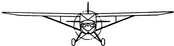
Fig. 313.—Airfoil section: N.A.C.A. 4412 is used on the Luscombe Model 50 two-place monoplane.
