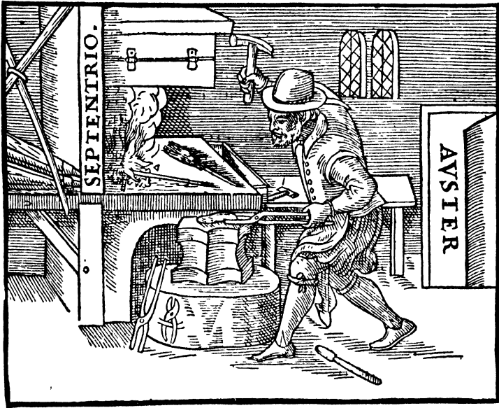
FIG 30 —Making a magnet by hammering iron in the N—S meridian (From Gilbert's De Magnete , 1600)
