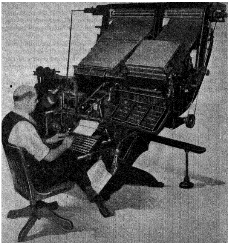
FIG. 2.—Proper position of operator at the keyboard. Body erect, hands level with elbows, and chair at convenient distance from the keyboard.
