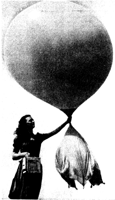
Fig. 19.8. Observer is ready to release balloon with parachute and radiosonde attached. (Courtesy U. S. Weather Bureau)
