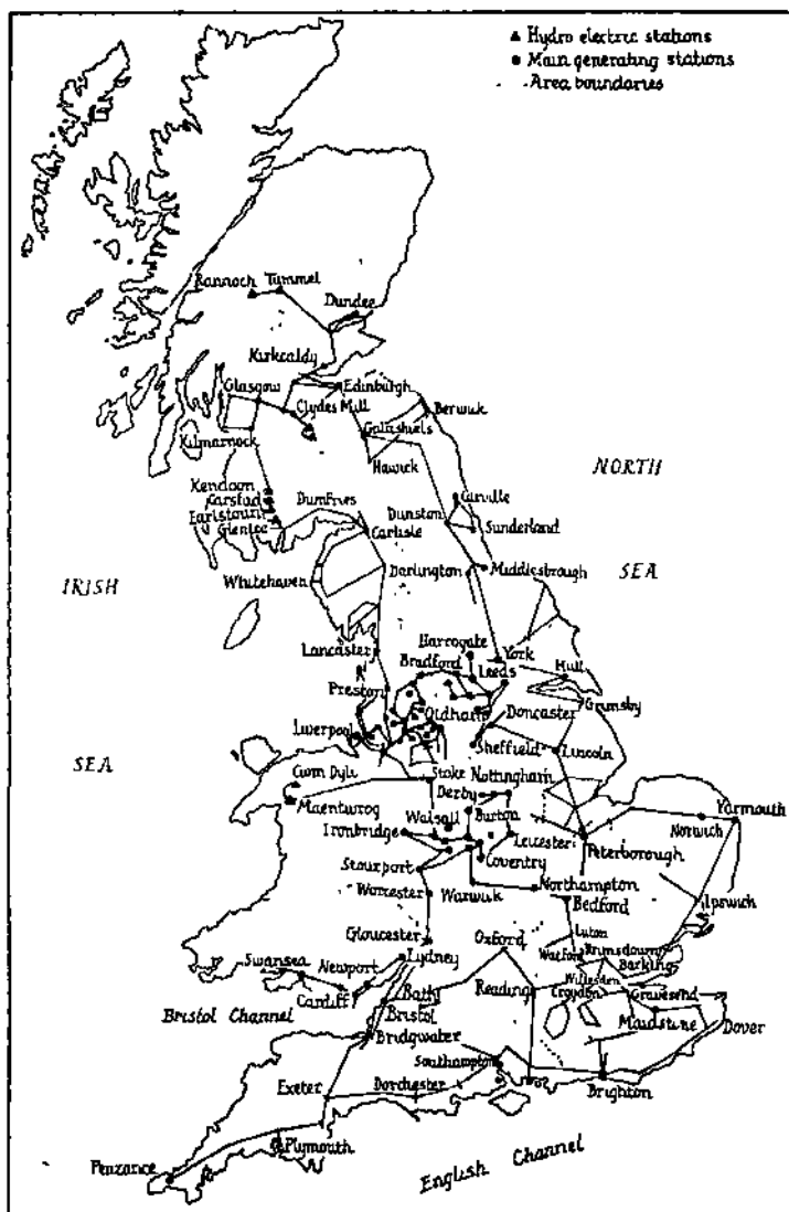
FIG. 56. TRANSMISSION LINES OF THE NATIONAL ELECTRICITY GRID Based on a map appearing in "The Times Electricity Supply Number," of December 5, 1933, by permission of the Central Electricity Board
