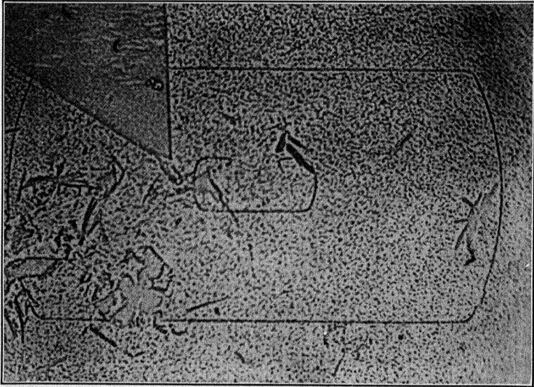
FIG. 10.14 Griffin's original (1950) phase-contrast micrograph of growth steps on a natural beryl crystal.
