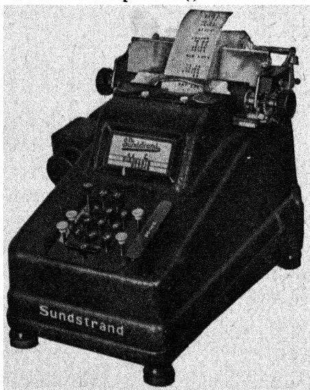
The machine illustrated above provides facilities for listing the figures as the calculations are being made
