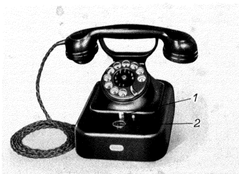
Station on a selective ringing system. 1 --- Tapping key 2 --- Busy indicator
