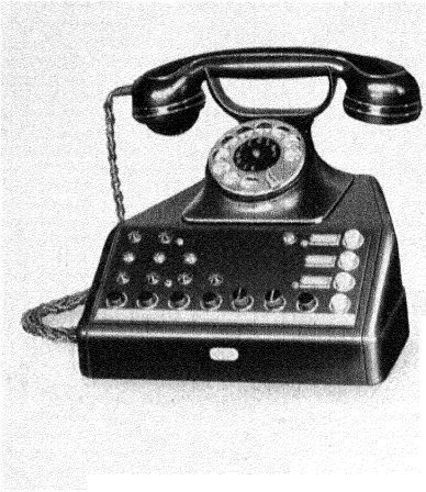
Principal's station for 1 exchange line, 1 extension line and 1 line to the secretary. Two switch-over keys and various keys for messenger calling, secretary calling and door locking.
