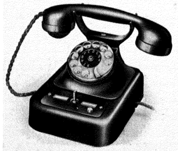
Main station of the Neha- exchange 1/4.
