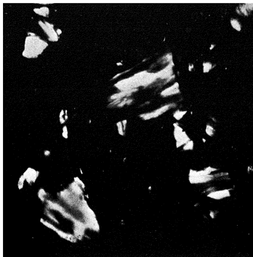
FIG. 8.—Annealed glass of composition 5\text{CaO} \cdot 3\text{Al}_2\text{O}_3 (crossed polars). ( \times 250 )
