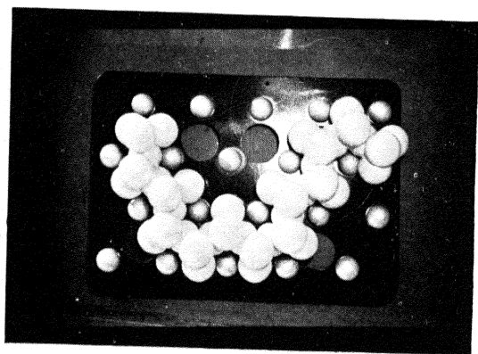
FIG. 3.—Photograph of model showing part of a metaphosphate ion adsorbed on calcite lattice.
