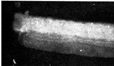
FIG. 3.—Quartz growing on surface of broken seed crystal. ( \times 20 )
