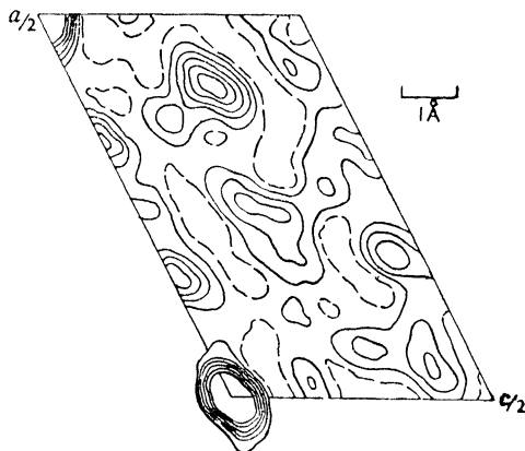
FIG. 187. Patterson function of \text{NaOH} \cdot 4\text{H}_2\text{O} , projected on (010)
