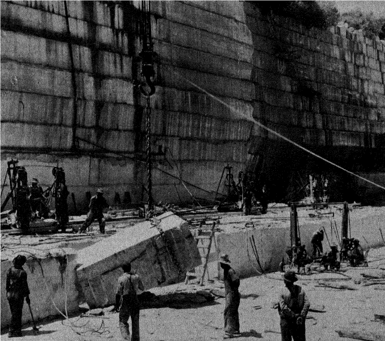
FIG. 36.—A marble quarry showing simultaneous hoisting, channeling and gadding operations. ( Courtesy of Georgia Marble Company. )
