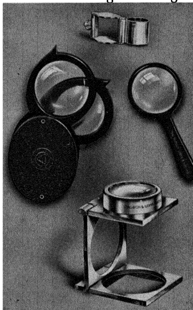
FIG. 15A. Types of Simple Magnifiers
