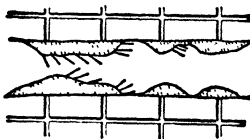
Fig 586. Miami Method, Horiz Sec through Stope, showing Drill Holes
