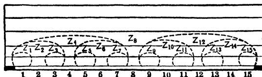
Fig 800 Effect of Extent of Excavation on Amount of Movement (Fayol)
