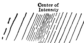
Fig 15 Sheeted Zone (Cross-section), showing Largest Number of Cracks at Seat of Heaviest Movement
