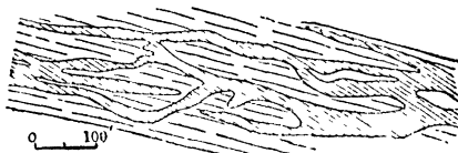
Fig 10 Irregular Replacement Orebody in Limestone (Showing Greatest Extent Parallel to Bedding Planes). Longit sec. After A. A. Blow
