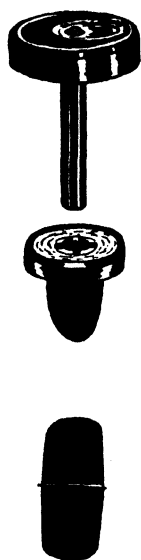
FIG. 16.—Types of stopper for Gerber's butyrometer.
