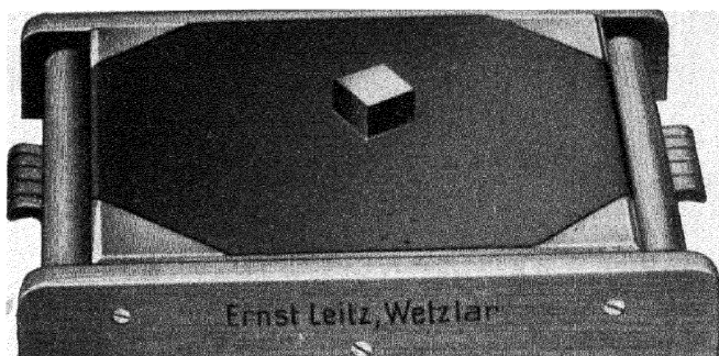
Fig. 66. —HAND POLISHING BOARD FOR THE PREPARATION OF METAL SPECIMENS
