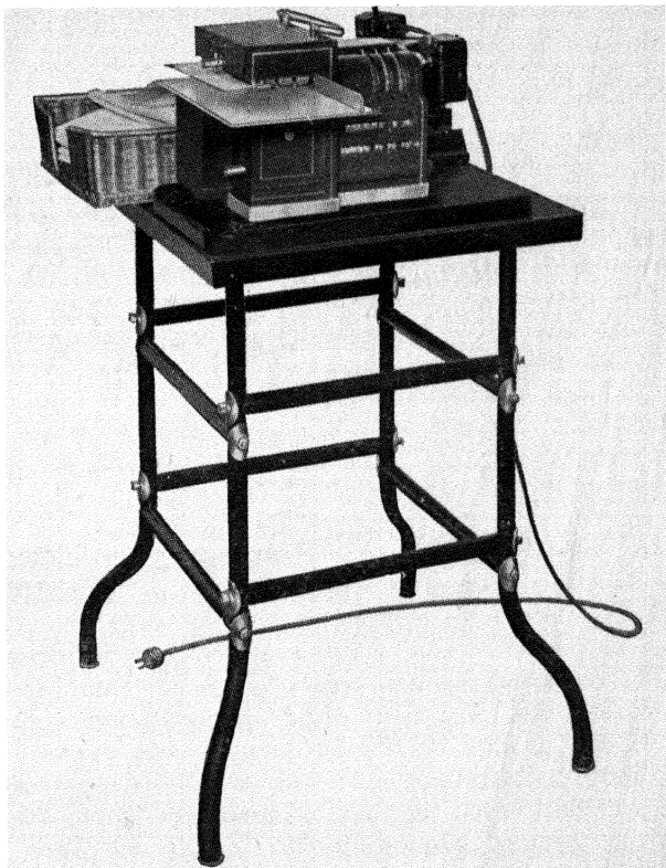
FIG 31 "MULTI-VALUE" UNIVERSAL FRANKING MACHINE
