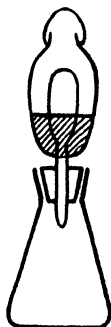
Fig. 43.—Meissl Ventilation Valve. Apparatus for permitting the \text{CO}_2 given off in Yeast-fermentation to escape. The water, however, which is given off in the form of vapour is retained.
