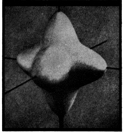
Figure 2. Elastic properties of iron crystals: the length of the vector from the centre of the model to any point on the surface is proportional to the rigidity modulus, the cubic axes of the crystal being indicated (Goens and Schmid 14 )
