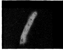
Figure 10. Focused Laue spot of an aluminium crystal made from the melt
