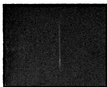
Figure 4. Focused Laue spot of a perfect single crystal of aluminium
