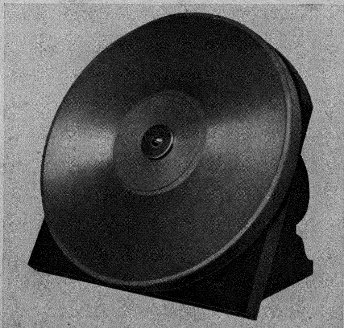
Fig. 128.—Wax record coated with graphite ready for electro-deposition of copper
