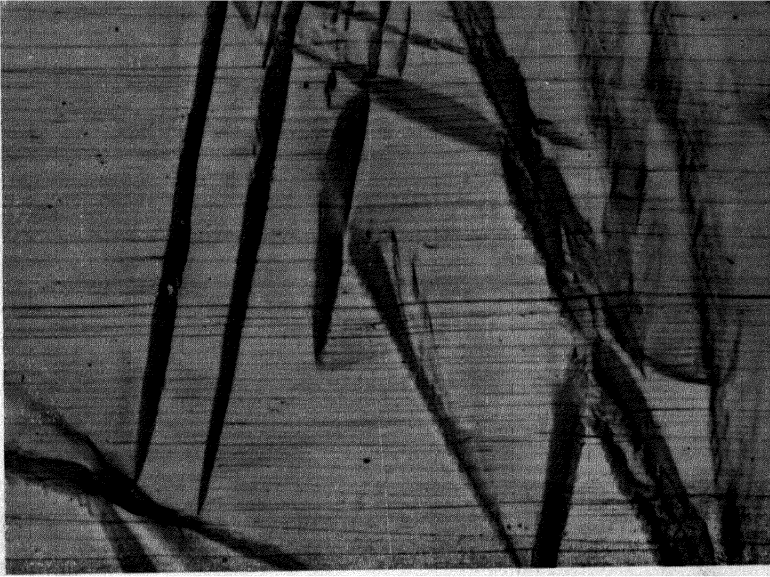
Figure 1. Martensite crystals in a large grain of a partially transformed alloy of iron-30 per cent nickel (polished and scratched before transformation and unetched). The distortion from the transformation has bent the scratches and tilted the surface (Magnification 150 ×)
