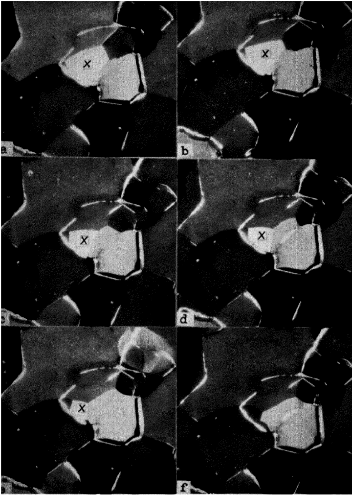
Figure 21. Grain growth in zinc observed with polarized light on a hot stage at about 200°C: the white grain marked X is gradually being consumed:
