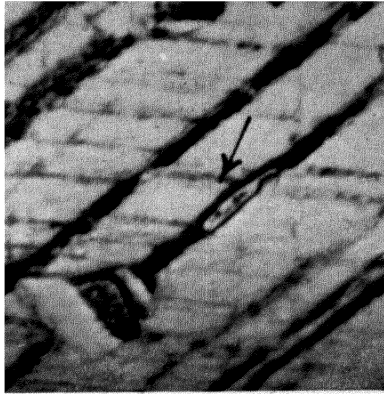
Figure 15. A small grain growing in a highly strained region (magnification 2000 ×)
