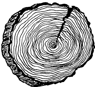
Timber cut across, showing rings, and crack during drying.
