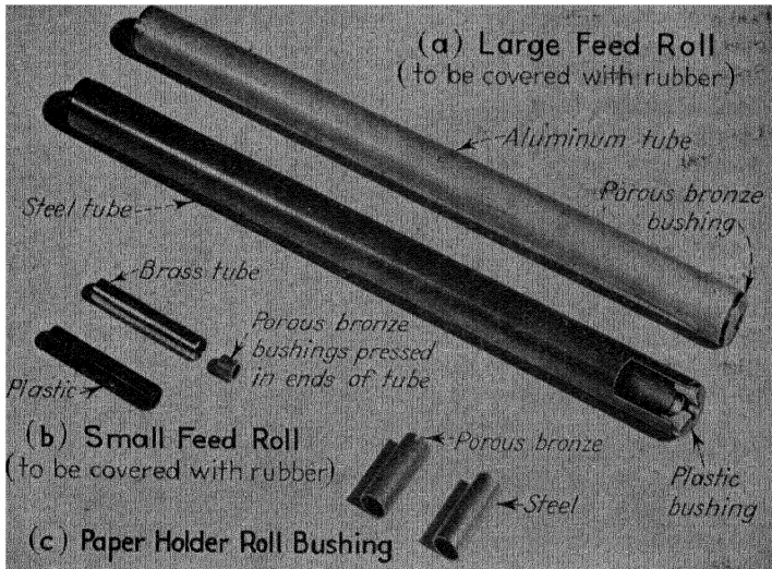
FIG. 93d.—Cellulose acetate plastic replaces porous bronze bushing in new Royal typewriter design.
