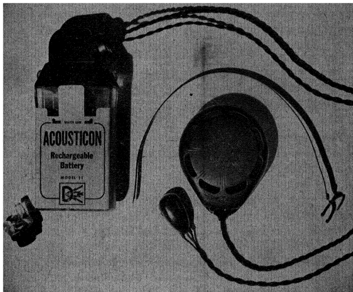
FIG. 4.—Wet-battery housing molded of polystyrene. Light weight, acid resistance, and good electrical characteristics were factors in the choice of material.
