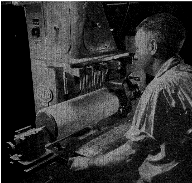
FIG. 53.—Drilling a molded-laminated tube on a multiple drill, eight holes at a time.
