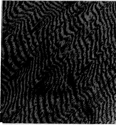
FIG. 50.—Electrodeposited Tin, scratch-brushed ( \times 140 ).
