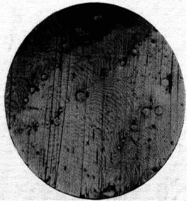
FIG. 46.—Ridged Effect associated with Grease Lines ( \times 25 ).
