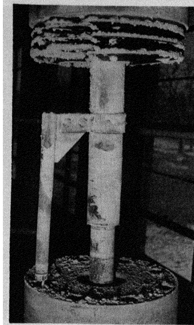
FIG. 2-28. View of EBR-II model tank fuel subassembly storage basket after removal from sodium directly into air. Location of basket in tank is shown in Fig. 2-22.
