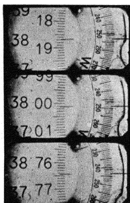
FIG. 14. Section of a current meter record during ten minutes. Left: number of revolutions of the blades. Right: compass readings; the pointer shows the direction of the current. (Magnified; width of original film 16 mm.)
