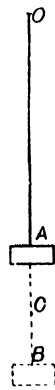
FIG. 72. lower end, when the mass is twisted round and released it oscillates to and fro round the wire as axis.
