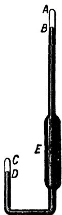
FIG. 118.—Bunsen's Apparatus for Determining the Raising of the Melting Point by Pressure.
